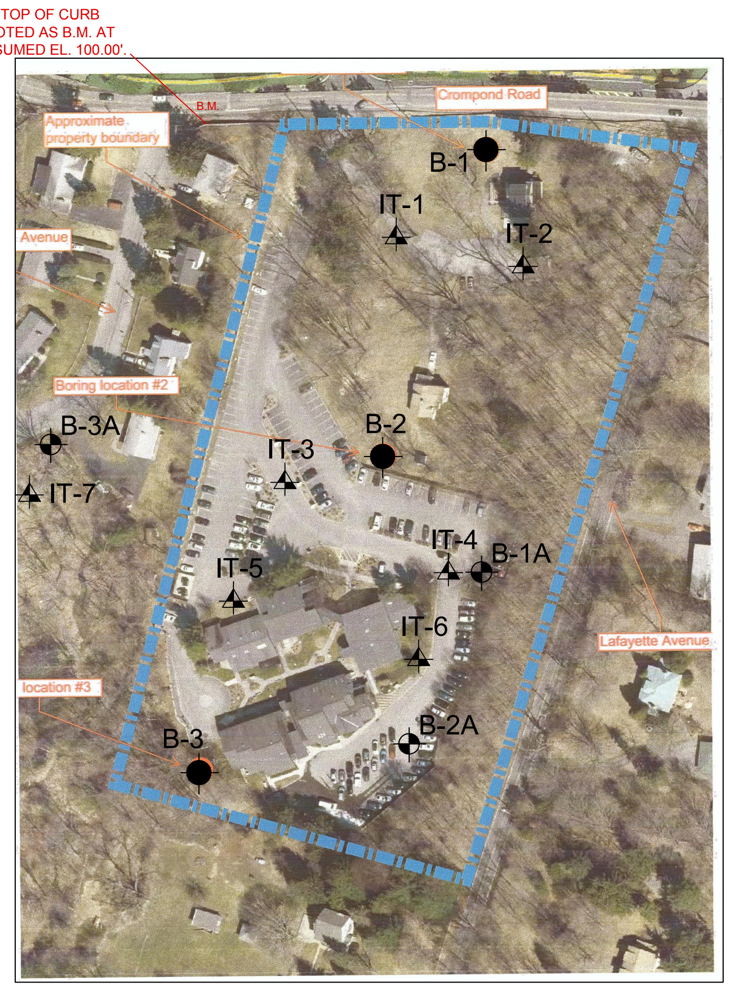
SOIL TEST BORING / INFILTRATION TEST LOCATION PLAN
